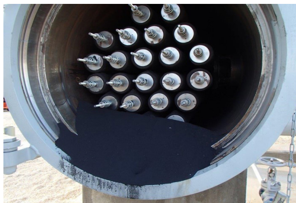
Figure 1. Uncaptured black powder built up in a conventional filter housing.
