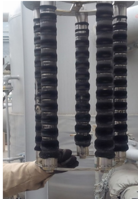
Right: Black powder contamination captured on the magnetic elements.
